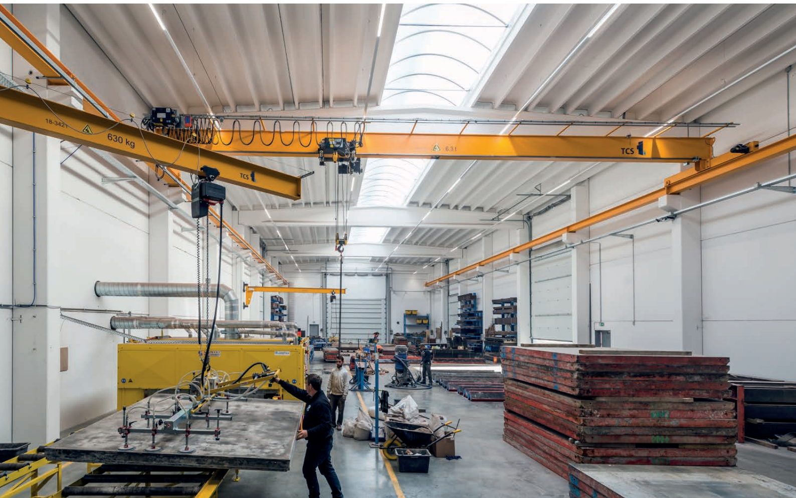
▲ Jib cranes are used to load panels into the cleaning machine.
