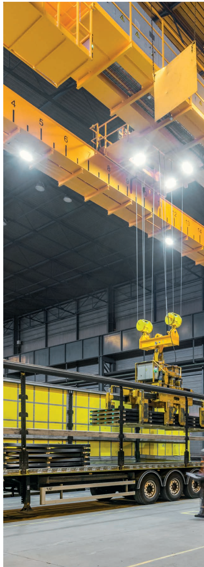
The dual hoist crane with frequency control improves stability when handling long sheets.
