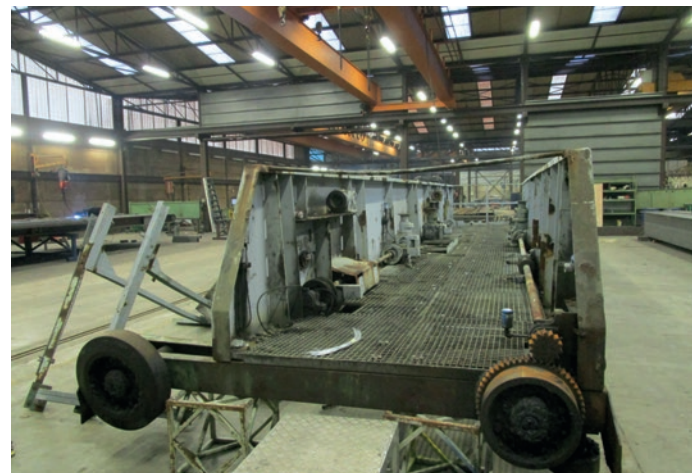
▲ The equipment was designed to carefully skim the oil accumulating at the surface of a 30m x 6m wastewater basin.
